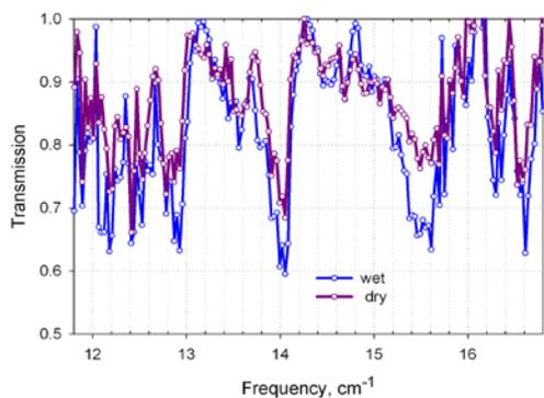
We have developed a new method of spectroscopic characterization of macro-molecular artificially designed structural elements of a modern nano-bio technology. The figure to the left shows the THz signature of artificial DNA nanocrystal, bio-molecular architecture built in the group of Prof. M. Norton, Marshall University, WV. (Submitted JPC (A), 2013, <http://pubs.acs.org>)
